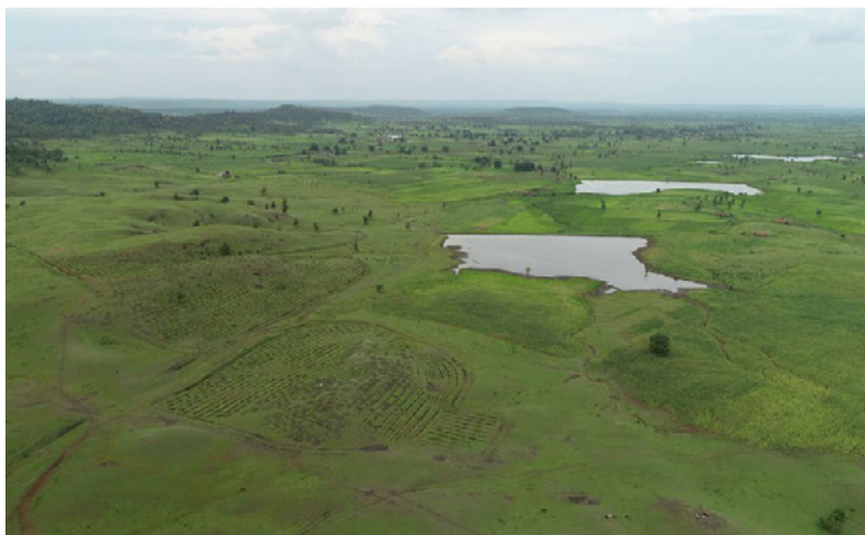
Image 2: continuous contour trenches collect water flowing downhill to be used in irrigation
